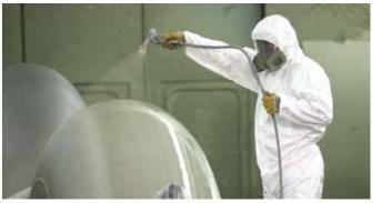
The Company is widely using modern equipment for applying liquid external polyurethane-based coatings on final products.
