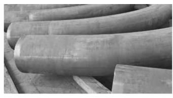
Buttwelding induction bends offered by TURUBODETAL OAO are manufactured using the following induction bending machines:
