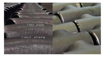
Pressed pipe fittings are produced in-house in the shop no. 2, equipped with 6 hot drawing machines, 2 hydraulic forging production lines, 3 presses for manufacturing pipe adapters and plugs.
